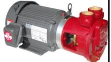
Model LR - 1", 1 1/2" and 2" NPT ports, 1800-3600 RPM, Flows to 80 GPM, 230' TDH. For direct drive applications
