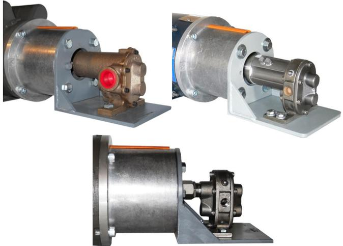
Our Direct Mount Adapter Kit will accommodate direct mounting all Model LOS, LOM, LOL/LOI, LOE/LOX and MOE/MOX gear pumps to any C-Face electric motor, frame sizes 56C, 143C, 145C (Up to 2 hp). We use a standard SAE pump mount adapter with our special bracket for a simple bolt on solution.
