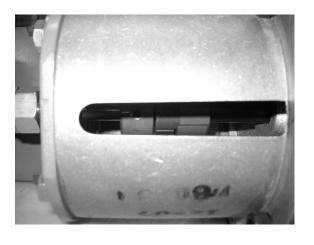
10) The shaft couplings should align/fit like pictured here to the left.
