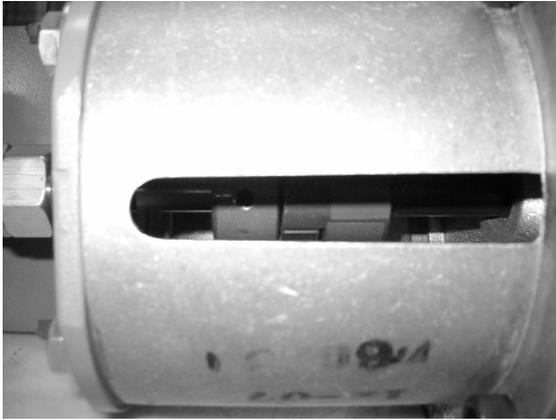
**10)** The shaft couplings should align/fit like pictured here to the left.
