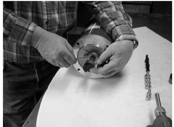
**2) Align main body of jaw style coupling with end of motor shaft. The shaft must not protrude into jaw cavity. Tighten coupling set screw securely.**
