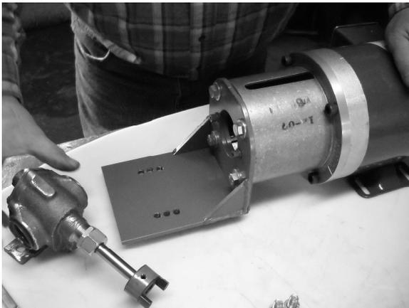
**8)** With the bracket and SAE mount fastened to the motor, install the rubber coupling spyder (element) into the motor coupling half.
