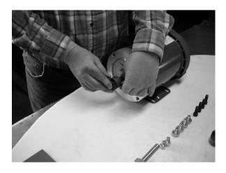
Align main body of jaw style coupling with end of motor shaft. The shaft must not protrude into jaw cavity. Tighten coupling set screw securely.
