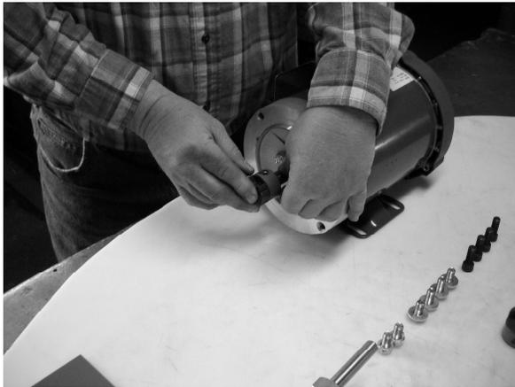
**1) Install correct coupling half on motor.**
