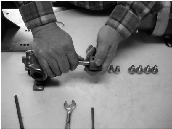
**4)** Install correct shaft coupling half on pump. Align main body of jaw coupling with end of shaft.
